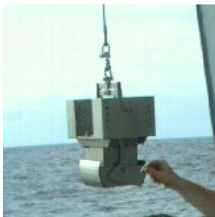
Figure B.7 The small box corer being deployed off the RV Southern Surveyor .
