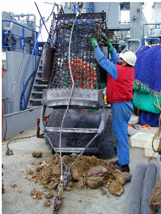
Figure B.8 The AGSO rock dredge and catch on the back deck of the RV Southern Surveyor .
