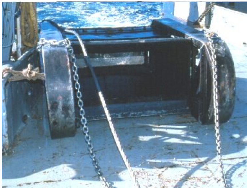
Figure B.5 “Sherman” the epibenthic sled, front view, on the back deck of the RV Southern Surveyor .
