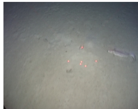
Figure 5.14 Examples of reference sit video frame grabs images for the four terrain types with depth of image shown below, laser dots at 200 mm*.
