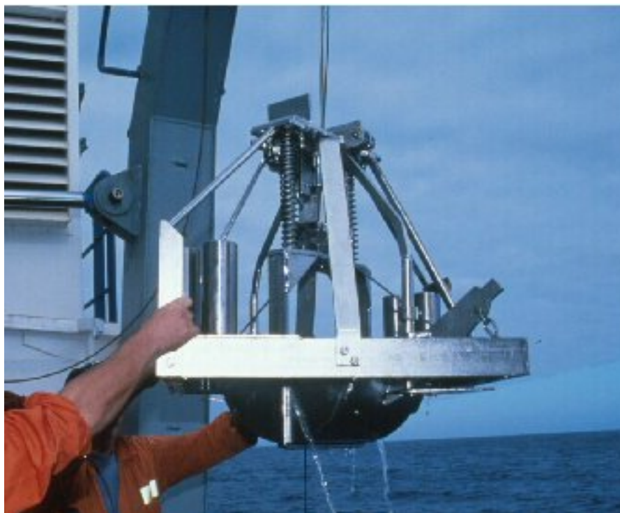
Figure B.6 The Smith-McIntyre grab being retrieved over the side of the RV Southern Surveyor .
