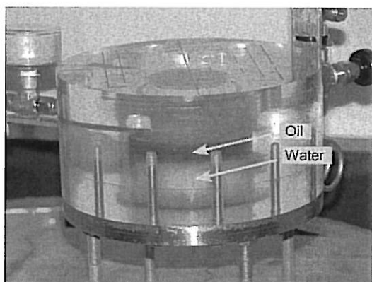
Figure 14. Separation between the oil and water in the pressure cell.
