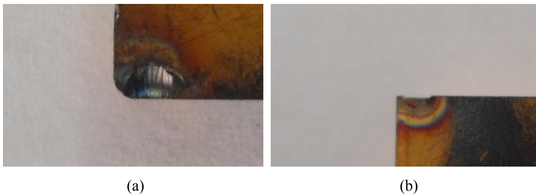
Figure 6.24: Collected chips after 7 min of uninterrupted turning operations under dry condition (a) connected arc chips, (b) a distinguishable pattern
