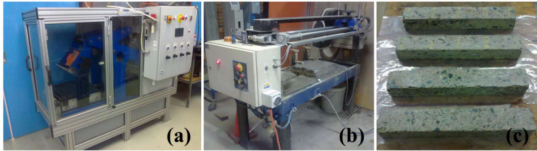
Figure 3.2: Manufacturing of small-sized beams: (a) a roller compactor used for making CTB slabs, (b) a cutting machine, and (c) prismatic beams cut from compacted slabs
