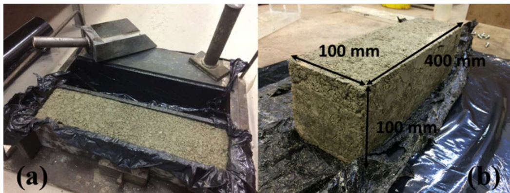
Figure 3.3: Manufacturing of large beam specimens: (a) a steel mould, and (b) a large-sized beam
