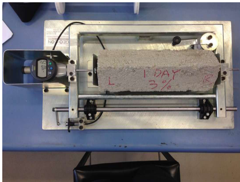
Figure 3.21: Horizontal comparator and shrinkage measurement of CTB specimen
