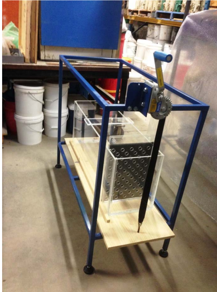
Figure 3-26: A view of the water section and winch in the manufactured apparatus
