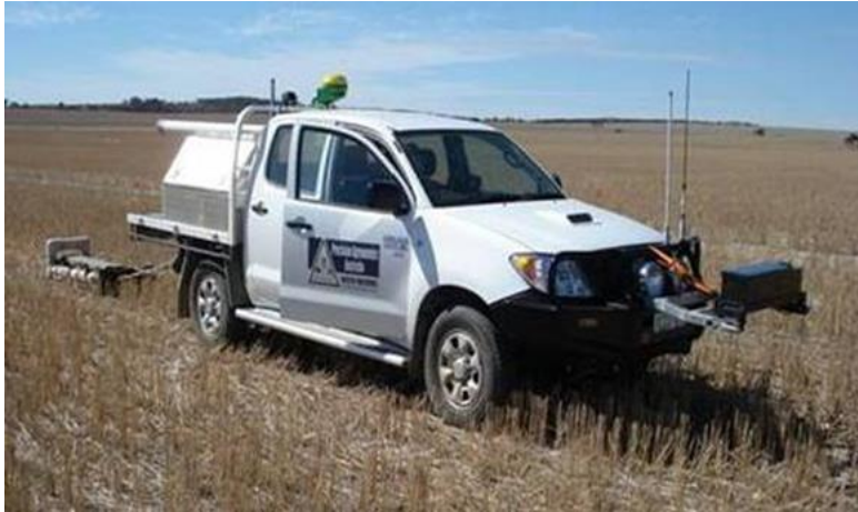
FIGURE 5.1: VEHICLE EQUIPPED WITH RADIATION SOLUTIONS RSX1 AND GEONICS DUALEM 21S SENSORS USED AT “MILROY”.
