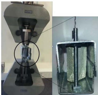
Fig. 2. Apparatus of pull-out test
