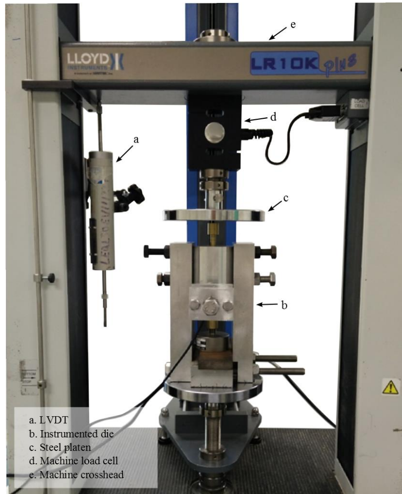
Figure 3.2: The assembled instrumented die on a universal tensile compression testing machine. A separate LVDT was attached to the crosshead to synchronise data between separate data loggers.
