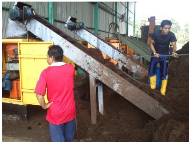
Figure 1.5: Matured EFB compost delivered with conveyor belt at the pelleting plant
