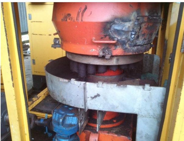
Figure 1.6: Processing EFB compost into pellet with pellet mill
