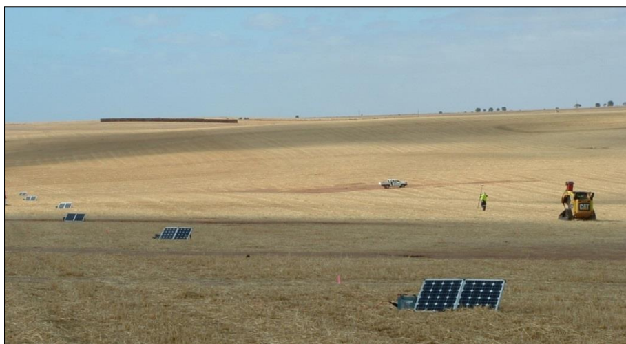
Figure 4-11: The solar panels were used to top up the batteries to increase effective shooting time.
