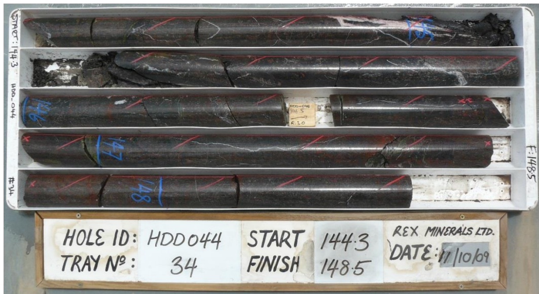
Figure 4-3: Core samples from the HDD-044 borehole (Tray length is 1 m and core diameter is approximately 45 mm).
