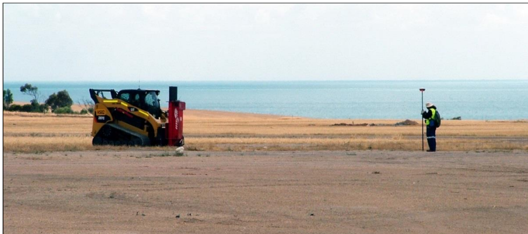
Figure 4-12: 375 kg free-fall weight drop was carried by a skid-steer to navigate to each shot point by a spotter.
