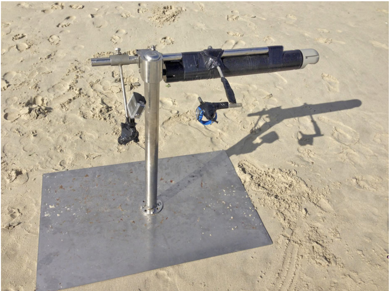
Figure 3.4 An apparatus designed to measure water currents while observing the suspension of drift algae samples. Included in the setup are a Nortek Aquadopp HR Current Profiler, a GoPro Camera and a stop watch.
