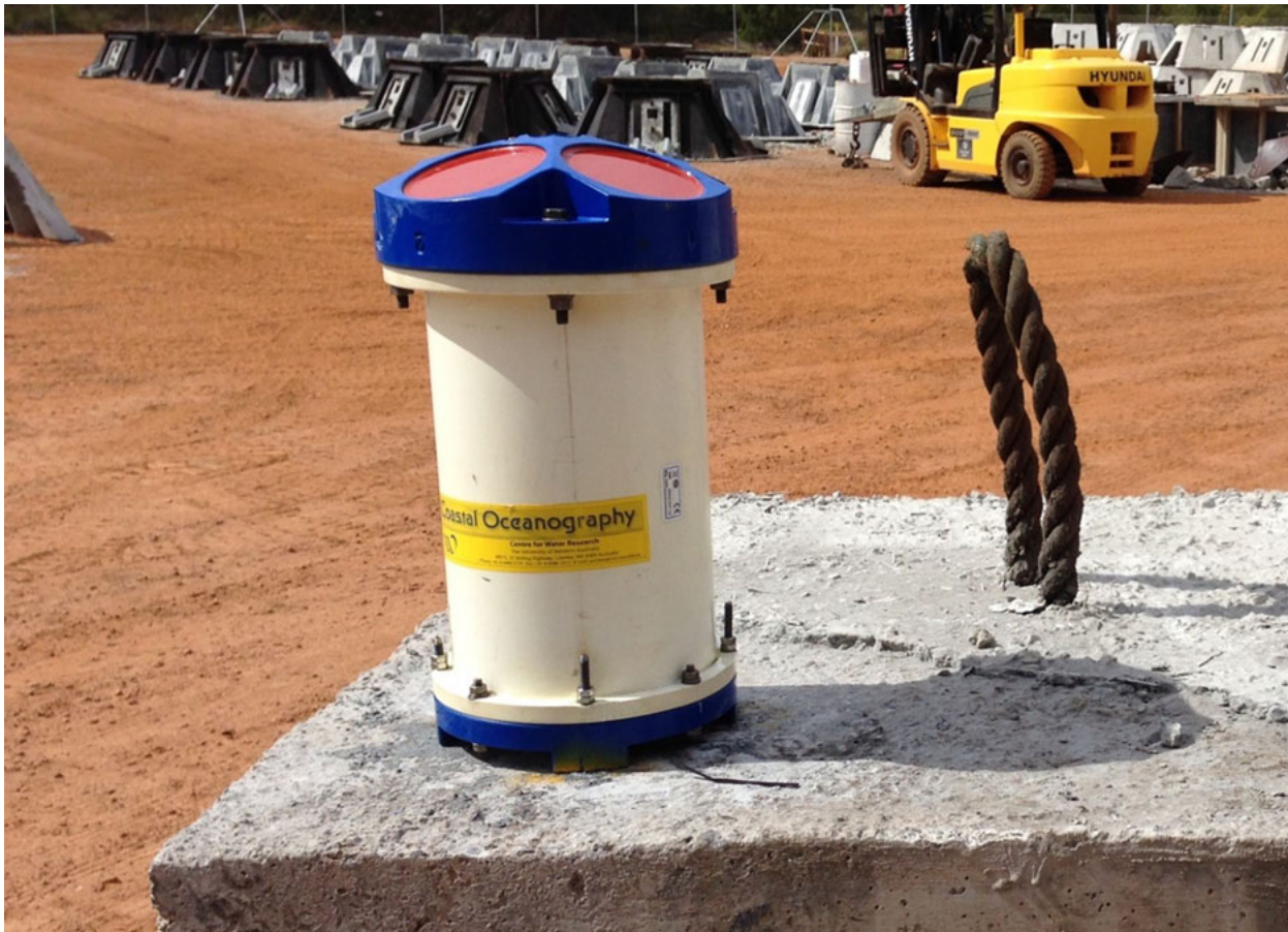
Figure 3.3 An ADCP attached to a concrete mooring at the OGA habitat construction yard
