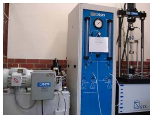
Fig.4 The GCTS STX-300 used for the CD triaxial compression tests
