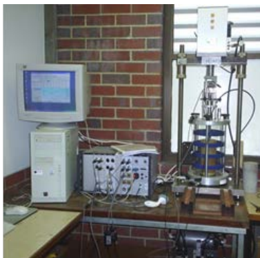
Fig.5 The UTM-14P used for static triaxial compression tests and repeated load triaxial tests
