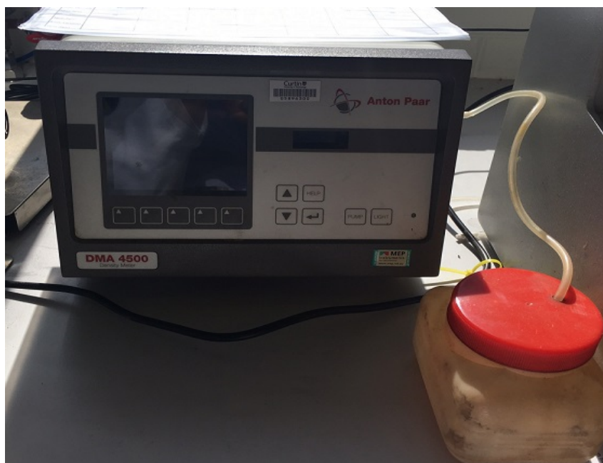
Figure 3-10. Density measurement using DMA 4500 Densitometer
