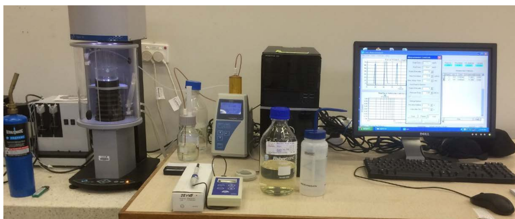
Figure 3-5. Equilibrium surface tension measurement using Wilhelmy plate method
