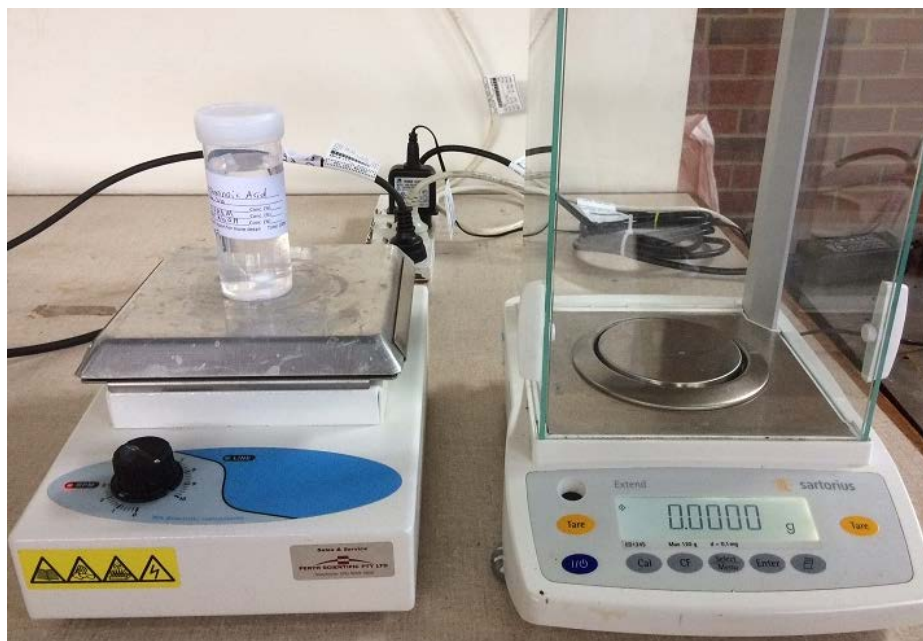
Figure 3-2. Nonanoic acid preparation using balance and magnetic stirrer
