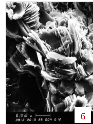
Figure 13. 1) Rock Classification using Folk (1974) for WR1&2 well; 2) Thin section showing Lithic Arkose from Whicher Range; and SEM photos showing 3) Quartz overgrowths, 4) Smectite pore lining, 5) detrital mica curved around framework grain 6) Kaolinite and illite infilling pore space. (from Lynsley, P., 1982 ; Poyton, D.J, 1982 and Fanning et al 1982)
