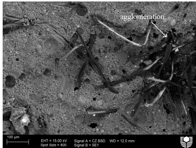
Figure 27: SEM showing agglomeration of short fibres in geopolymer matrix (Alomayri et al. , 2013a).
