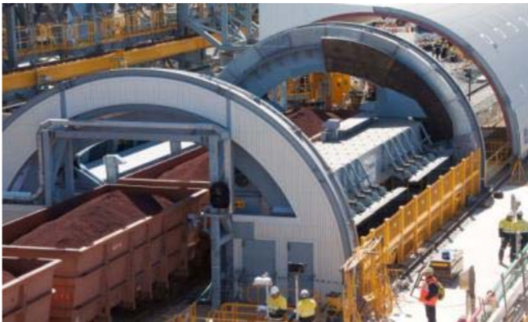
Figure 1.6: A car dumper operating at the port (Rio Tinto, 2013)
