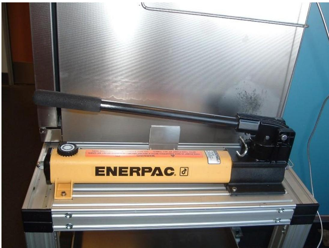
Figure 3.5 Enerpac hand pump pumps which is rated for pressure up to 2557 Bar
