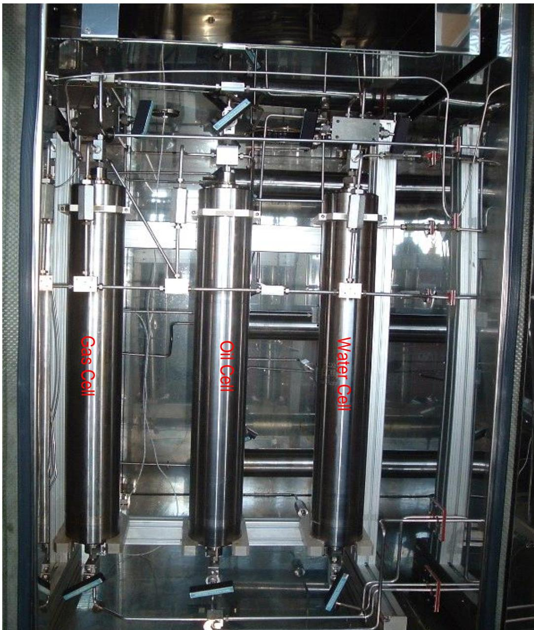
Figure 3.6 Gas, oil and water high-pressure vessels
