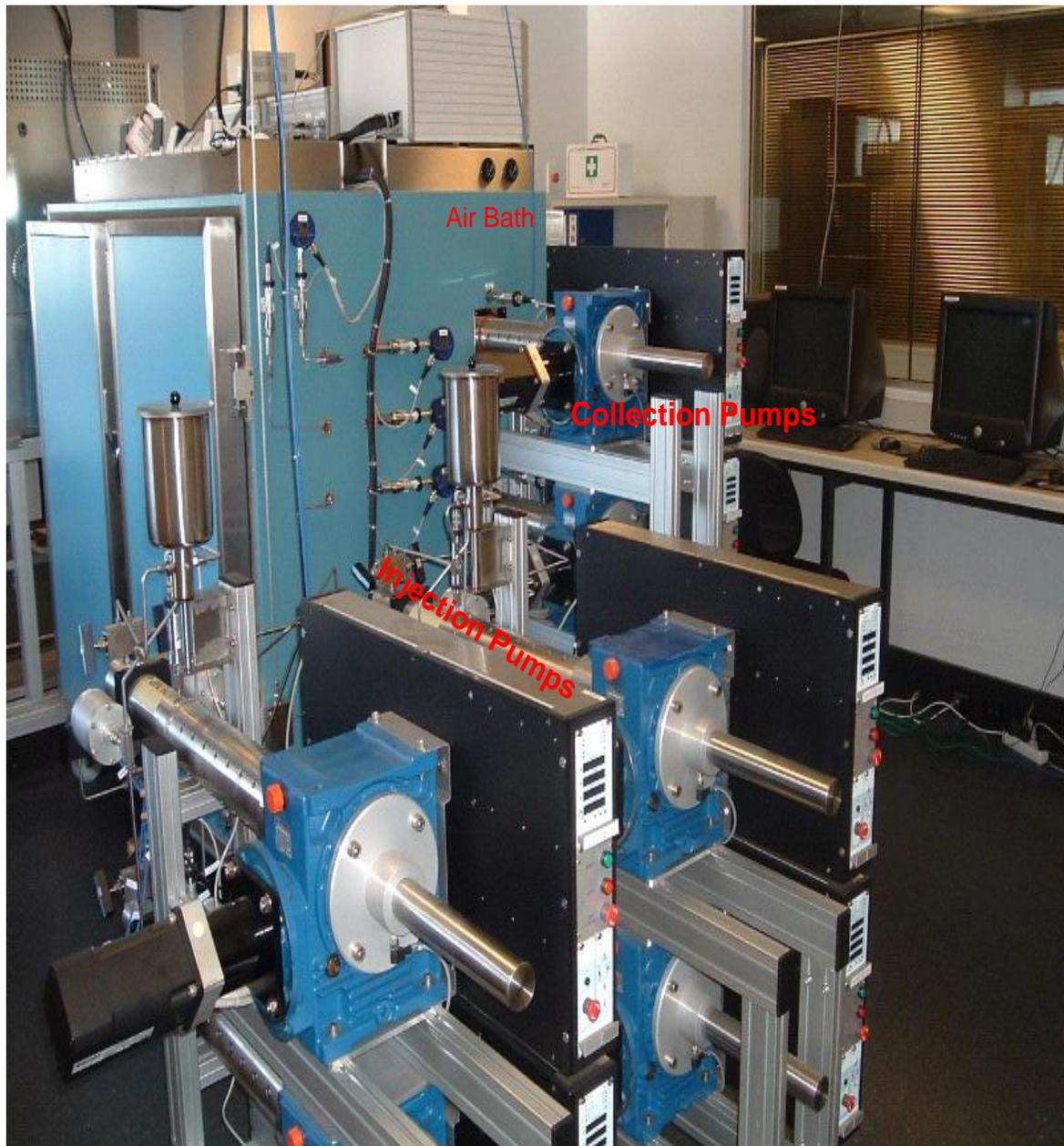
Figure 3.1 The three-phase core-flooding apparatus
