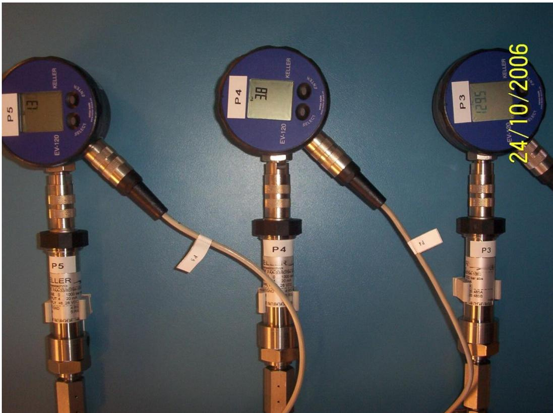
Figure 3.11 Pressure Indicators and Transducers
