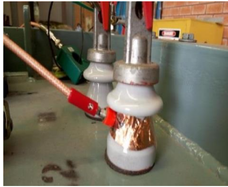
Figure 6.3. Capacitive coupling mounted on bushing
