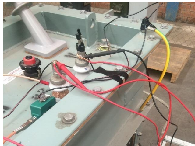
Figure 6.5. Signal injection and output measurement
