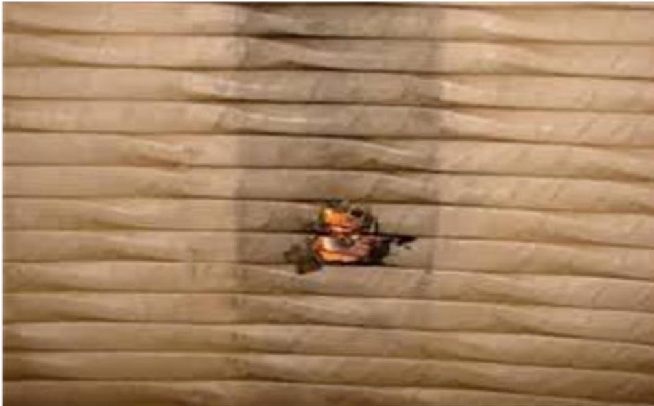
Figure 2.6: Inter-turn short circuit fault.
