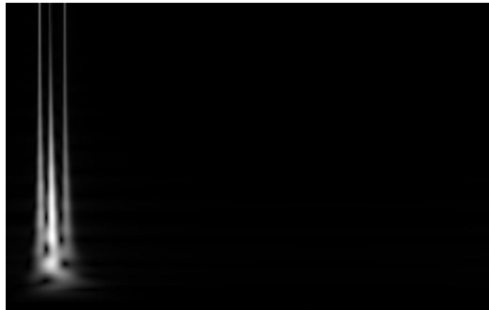
Figure 5.2. Intensity image derived from transformer output current time frequency contour
