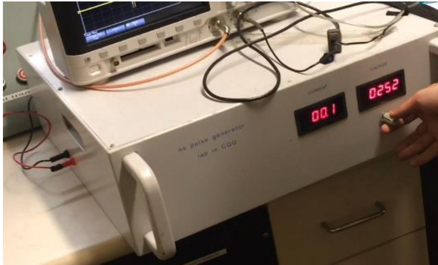
Figure 6.2. Nanosecond impulse generator
