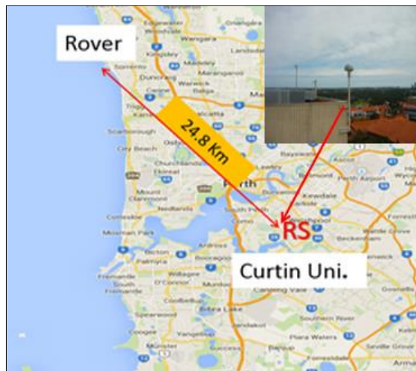
Figure 3.3: Location of GNSS observation station and reference station at Curtin University
