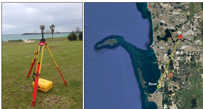
Figure 3.4: The static GNSS station setup at Kwinana Beach in Western Australia
