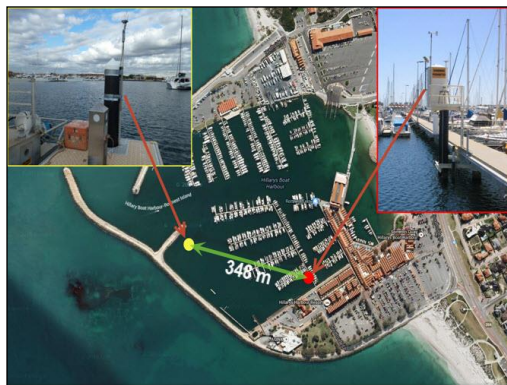
Figure 3.2: Hillarys tide gauge (red dot) and GNSS observation stations (yellow dot) (Fugro, 2014)
