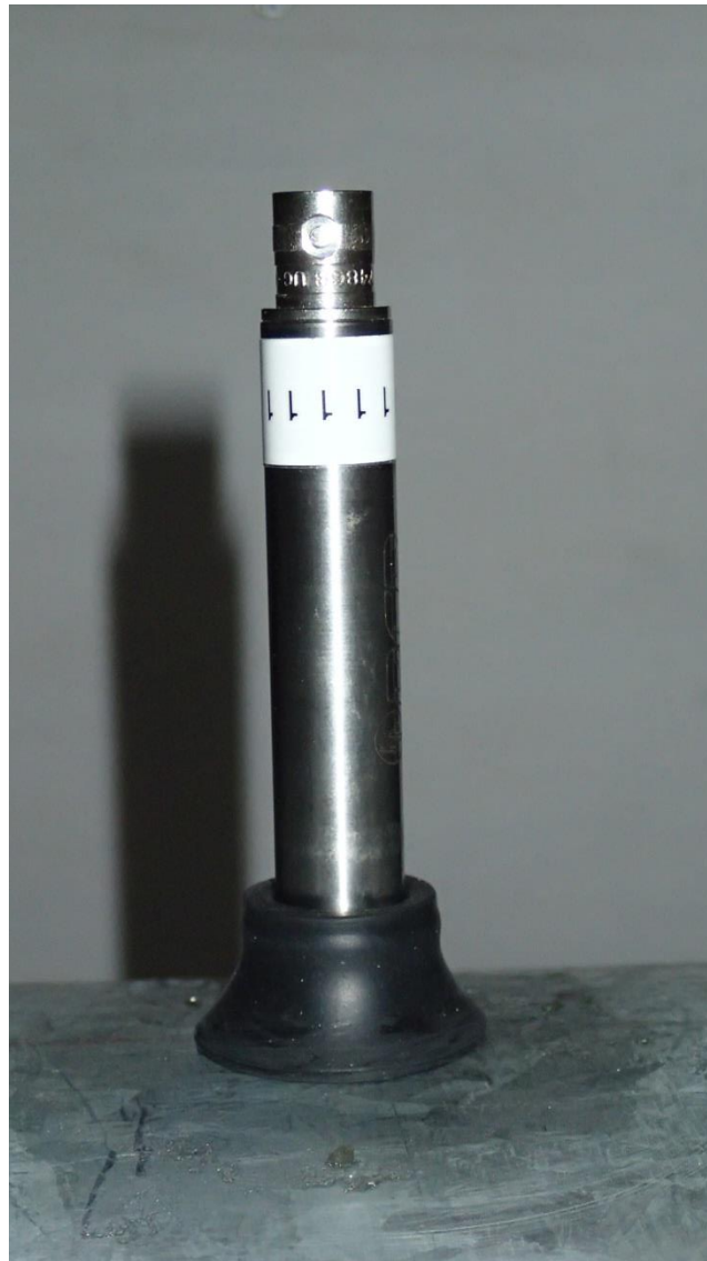
Figure 9.4 Microphone and Preamplifier in Grommet, External View
