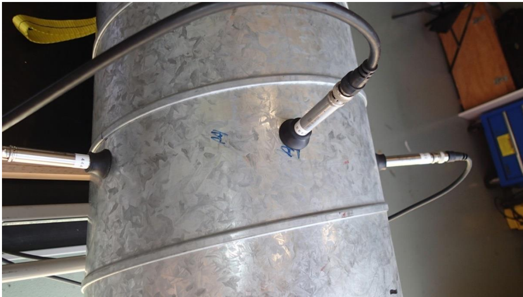
Figure 9.25 TL Bench, Microphone Matching Layout
