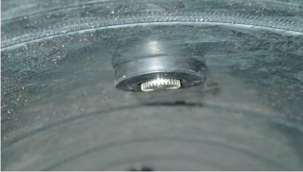
Figure 9.5 Microphone in Grommet, Internal View
