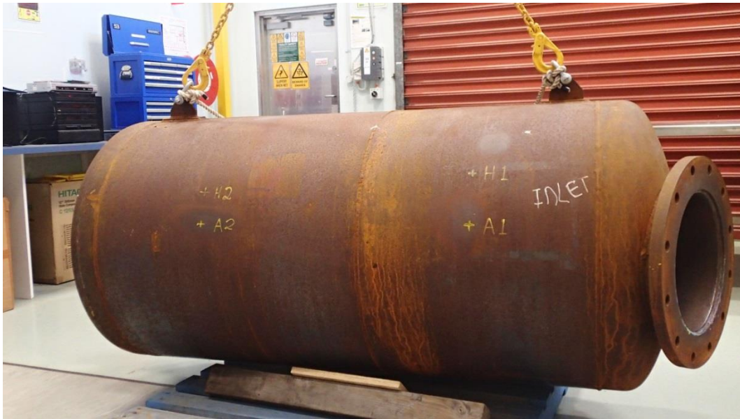
Figure 11.2 Muffler LMM, Ring Mode Locations, Data Sets TJuly01 and TJuly02
