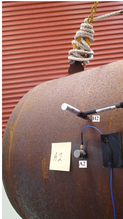
Figure 11.4 Muffler LMM, Ring Mode Locations, Outlet Side, Data Set TJuly02
