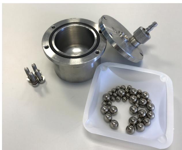
Figure 2.3: A 50 mL 316 stainless steel ball-milling canister with and balls sized at 10 mm and 6 mm.
