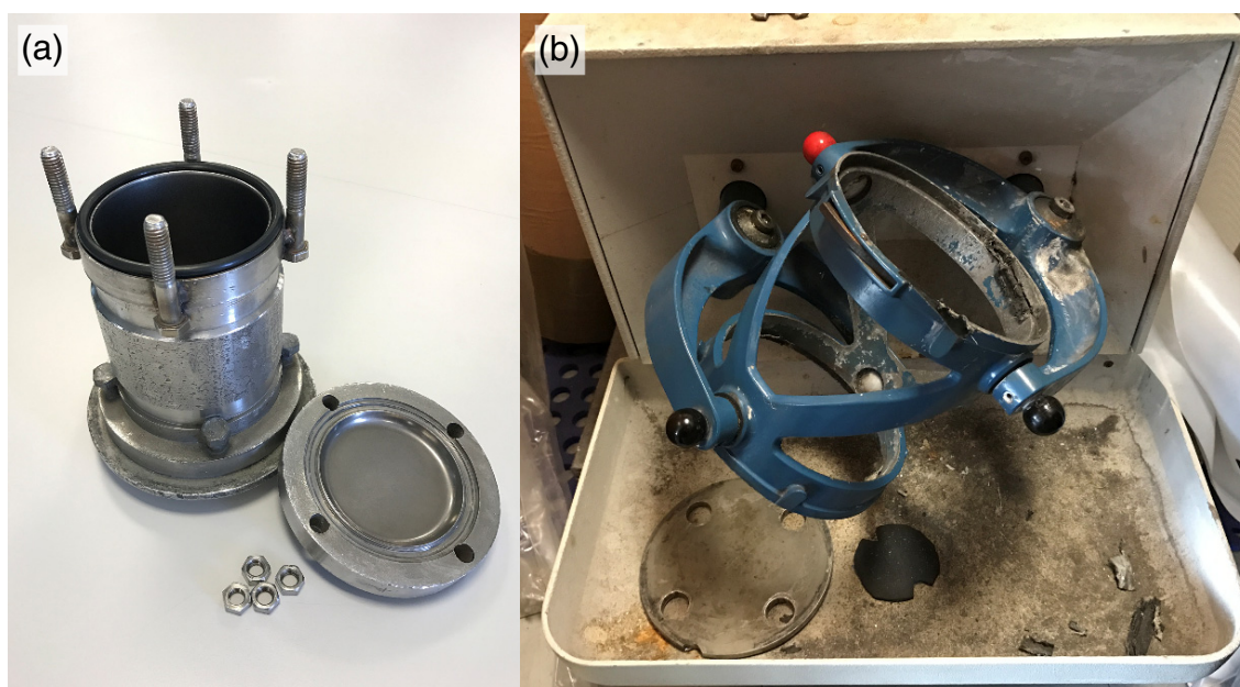
Figure 2.4: (a) A custom made 650 mL 316 stainless steel ball-milling canister and a (b) Glenn Mills Turbula T2C shaker-mixer (New Jersey, USA).
