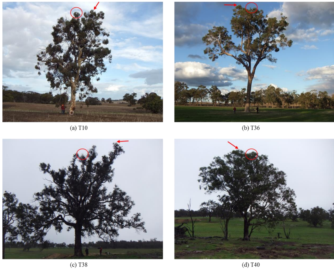
Figure 5.1.11: Examples of how the rangefinder can record a tree top point that is not the real highest point of the tree.
