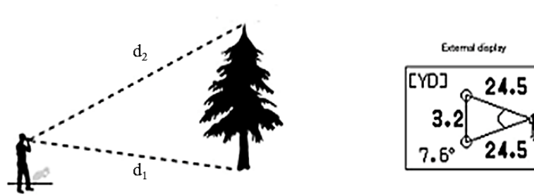
Figure 4.2.3: Height and depth measurement using the 2-point height measurement method as shown by the external display of the rangefinder. The distance from the rangefinder to the base and top of the target is denoted by d_1 and d_2 .
