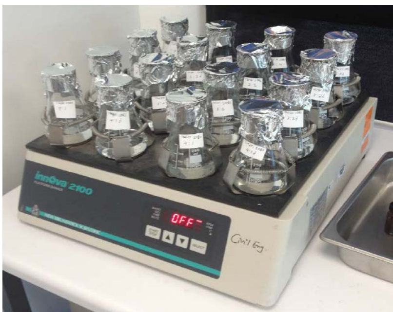
Figure 7.1: Experimental setup for surfactant enhanced PAH solubilisation
