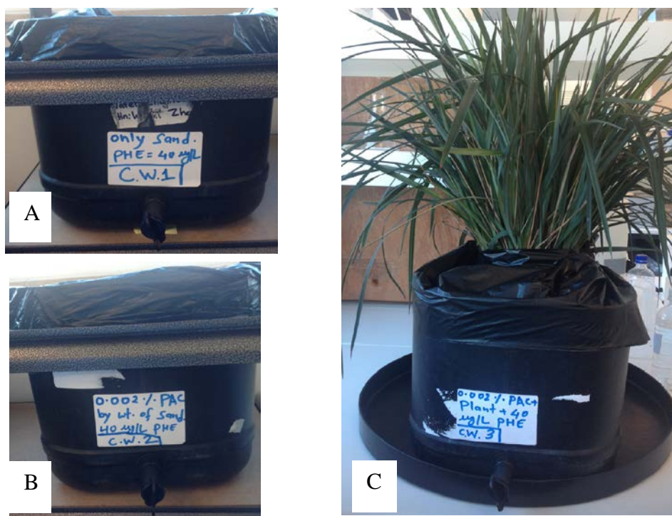
Figure 8.4: CWs with different media. (A): CW with sand media, (B): CW with sand and PAC, (C): CW with sand, PAC and plant
