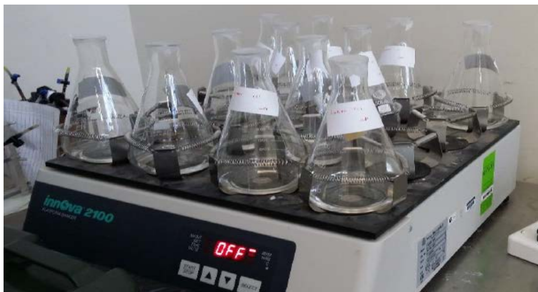
Figure 5.1: Batch experimental setup for PAH solubilisation with organic solvent
