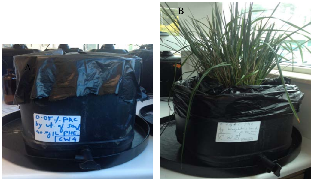
Figure 8.6: CWs with 0.05% PAC by weight of sand. (A): Without plant, (B): With plant
