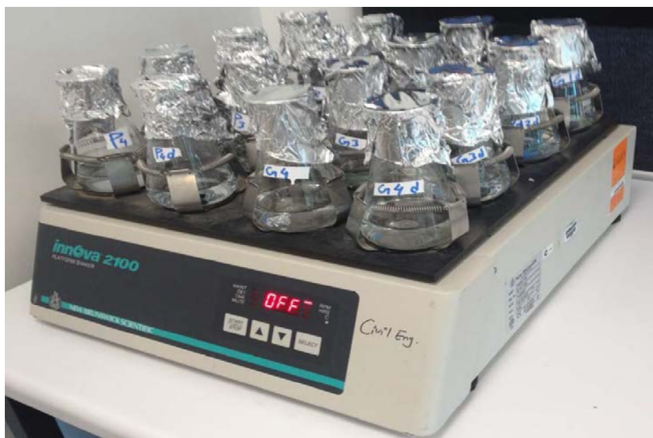
Figure 4.1: Batch test for adsorption of PAH with PAC and GAC
