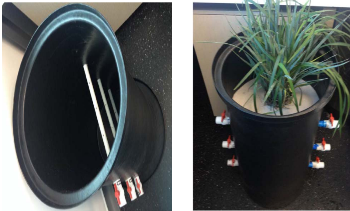
Figure 8.5: CW setup to study effect of depth in PAH remediation. (A): Porous pipes fitted at different depth, (B): CW after feeding bed materials
