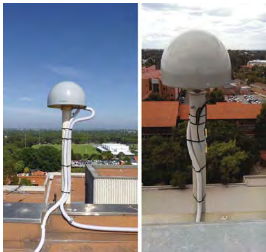
Fig. 1 CUCC (left) and CUBB (right) stations at Curtin University equipped with JAVAD TRE_G3TH_8 receivers, connected to TRM59800.00 SCIS antennas
