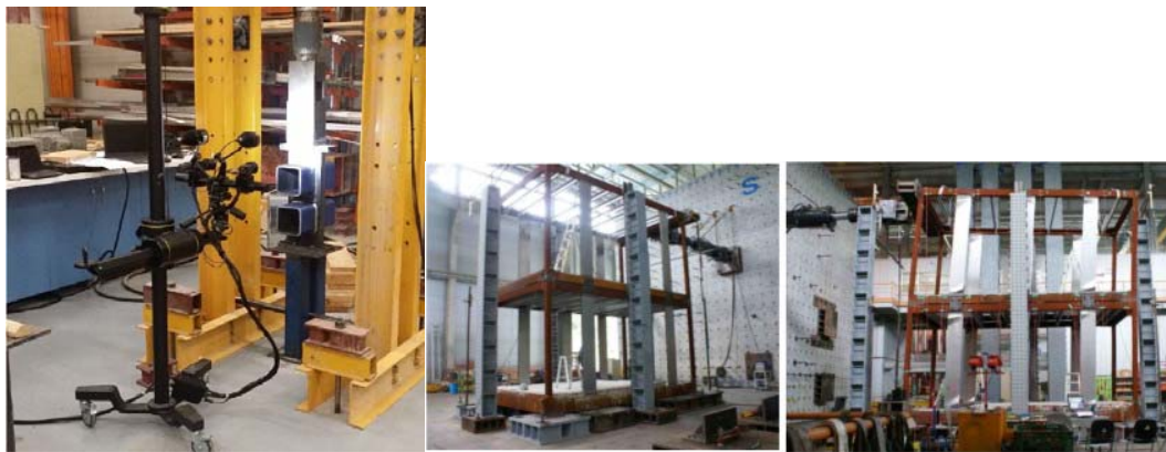
Figure 9. (L) Shear force load testing of connection with contactless strain measurement system [17], (R) Racking test of complete frame [55]
