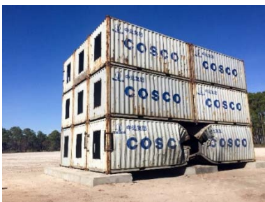
Figure 8. Expeditionary CONEX testing for progressive collapse [104]
