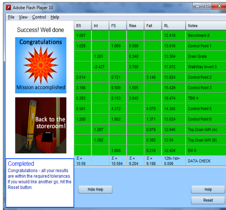
Figure 3b: Interface of the simulation tool after computations
