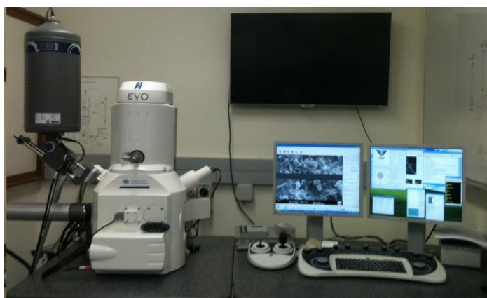
Fig. 4.4 Testing Machine used for SEM/EDS Analysis
