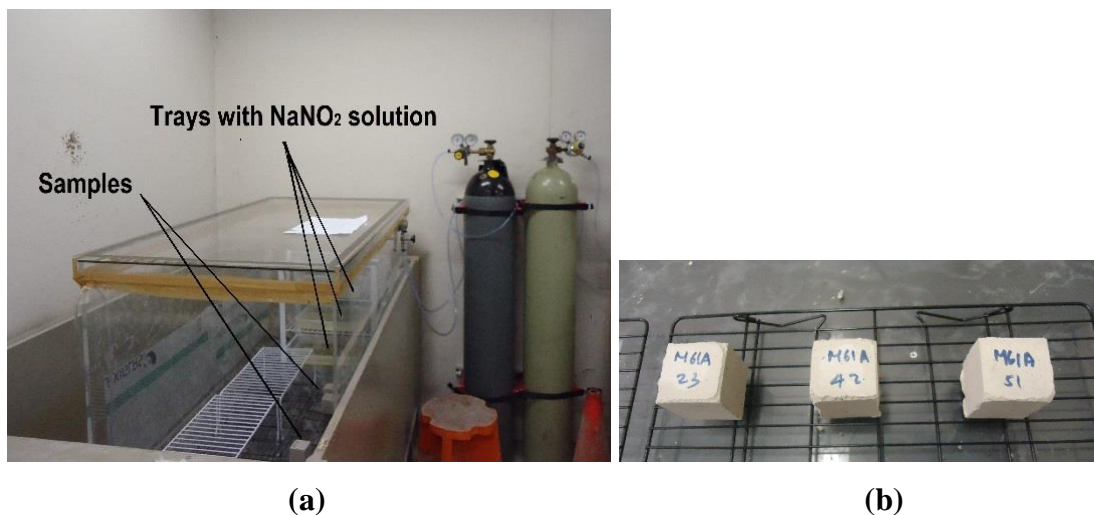
Fig. 5.4 Carbonation Test (a) Carbonation Chamber; (b) Samples kept on a ‘cake tray’ inside the chamber
