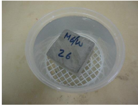
Fig. 5.2 NaCl Test: Sample with the container with NaCl solution
