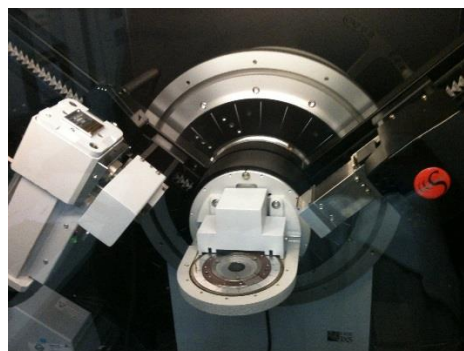
Fig. 3.6 A Sample Placed in XRD Testing Machine
