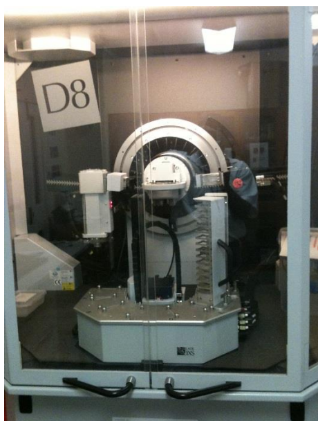
Fig. 4.3 Testing Machine used for XRD Analysis
