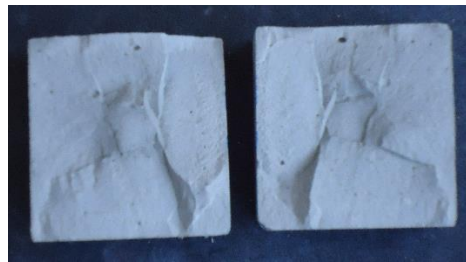
Fig. 5.20 Split sections of fully carbonated sample of HVFA mixture C3
