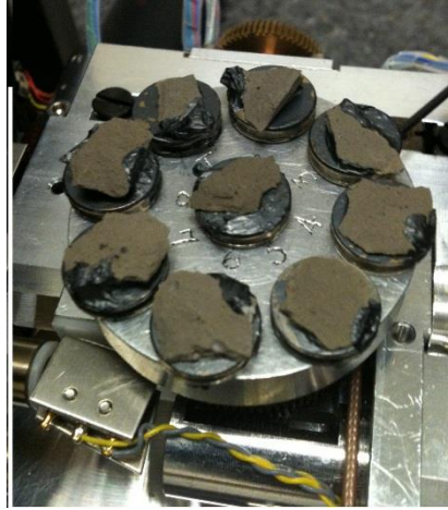
Fig. 3.7 Samples placed in SEM Testing machine
