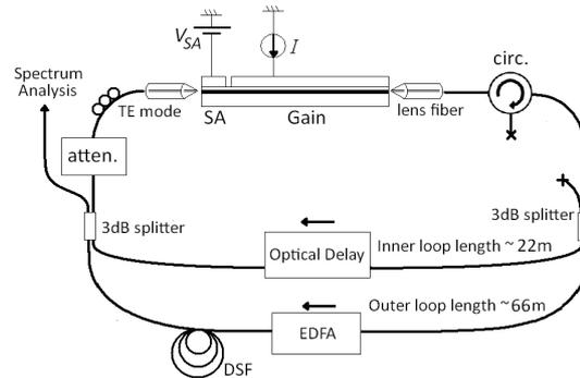
Fig. 1. Experimental configuration of the dual loop optoelectronic oscillator. (SA: saturable absorber, circ.: optical circulator, DSF: dispersion shifted fiber, atten.: optical attenuator).
