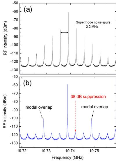
Fig. 2. (a) Uncorrelated composite cavity length resulting in large supermode noise resonances, and (b) optimized composite cavity length resulting in supermode noise suppression.
