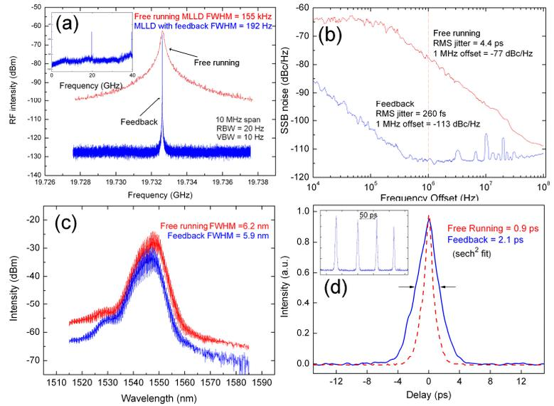
Fig. 3. Comparisons of free running MLLD performance and dual loop feedback performance in (a) the RF spectrum, (b) SSB phase noise, (c) optical spectrum, and (d) second harmonic generation (SHG) autocorrelation.
