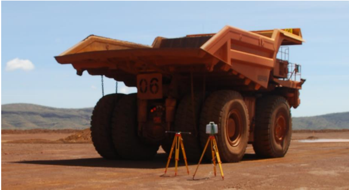
Figure 1: Laser scan of pavement deflection in progress with Komatsu 830E haul truck
