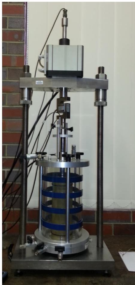
Figure 2: Triaxial testing laboratory setup.
