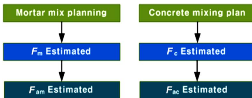
Figure 15. Estimation steps of F_{am} and F_{ac} from F_m and F_c .
