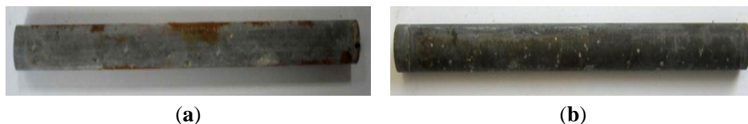
Figure 10. Appearance of reinforcing steel corrosion at the chloride ion concentration of 2.4 kg/m 3 and inhibitor molar ratio of 1.2. (a) Lithium nitrite inhibitor (LiNO 2 ); (b) Amino-alcohol inhibitor (DMEA).
