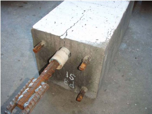
Fig. 3 (a) : Geopolymer concrete specimen
