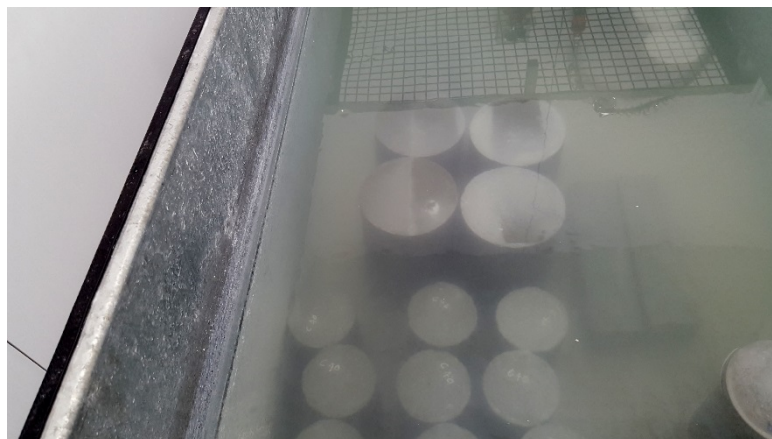
Figure 6-4: Concrete specimen curing under lime saturated water.
