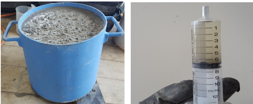
Figure 6-6: Bleeding test and bleed water collection.
