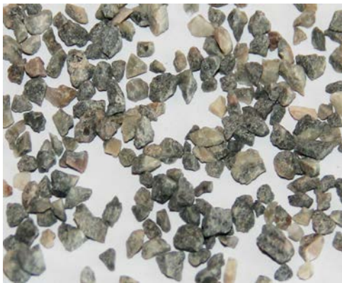
A – Retained on 1.18 mm sieve
