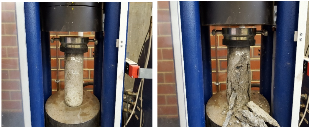
Figure 6-7: Compressive strength tests and failure of failure a specimen.
