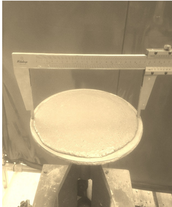
Figure 5-4: Measuring the flow of mortar.
