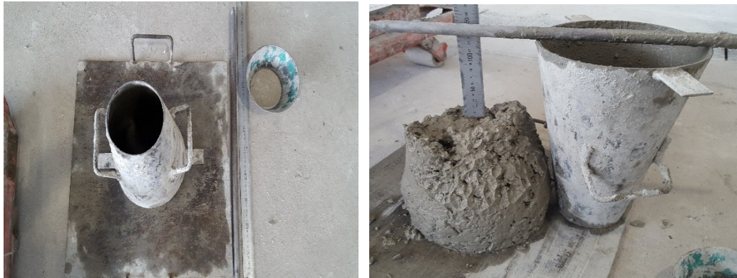
Figure 6-5: Workability test and measuring the slump of concrete.
