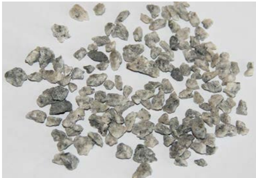
A – Retained on 2.36 mm sieve
