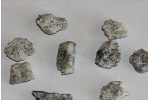
A – Retained on 6.7 mm sieve
