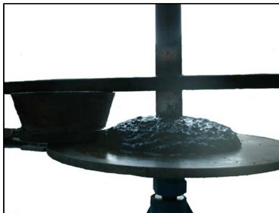
Figure 5-3: Measuring the slump of mortar.
