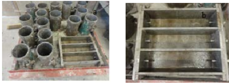
Figure 6-1: Moulds ready for casting.
