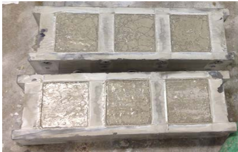
Figure 5-2: Mortar in mould after compaction.
