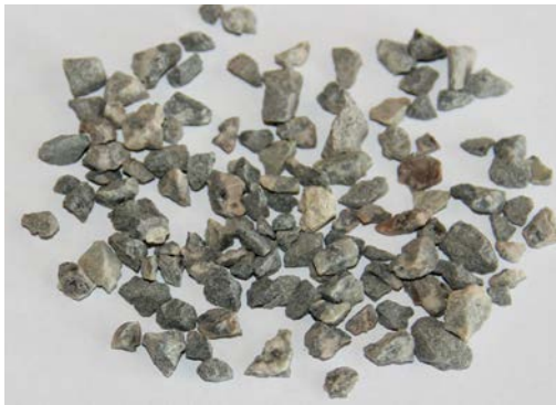
C – Retained on 2.36 mm sieve
