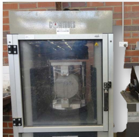
Figure 6-8: A sample subjected to indirect tensile strength test.
