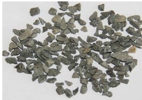
B – Retained on 2.36 mm sieve
