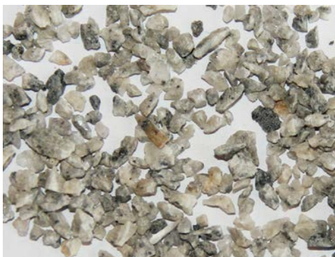
C – Retained on 1.18 mm sieve
