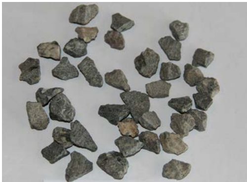
A – Retained on 4.75 mm sieve
