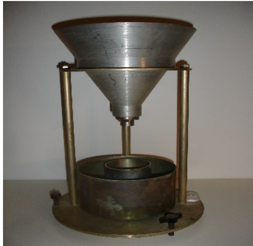
Figure 4-1: New Zealand flow cone test of fine aggregates.
