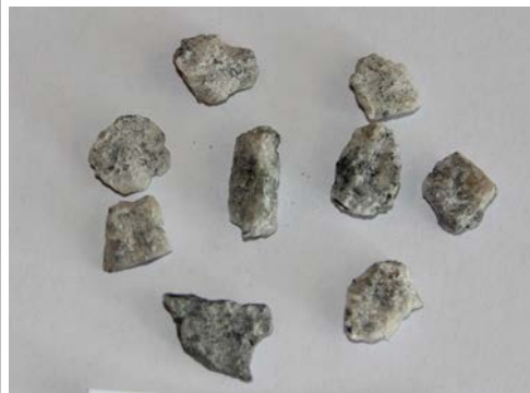
C - Retained on 4.75 mm sieve
