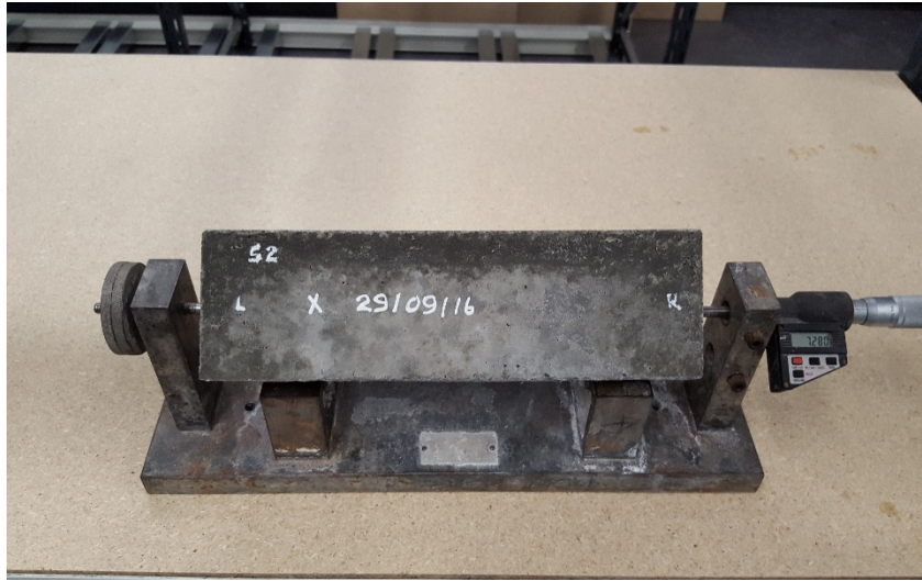
Figure 6-9: Length measurement by a horizontal length comparator.
