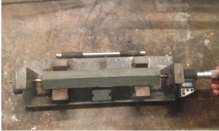
Figure 5-5: Measuring the expansion by using the comparator.
