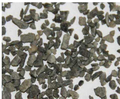
B – Retained on 1.18 mm sieve
