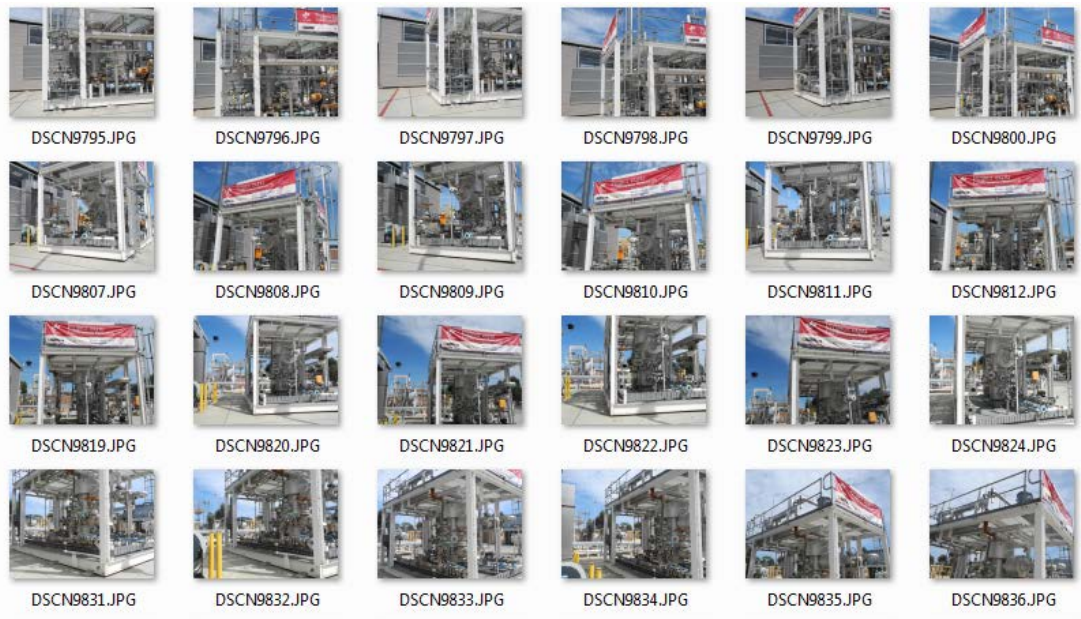
Figure 4.5. Photos used in the 3D reconstruction of the module
