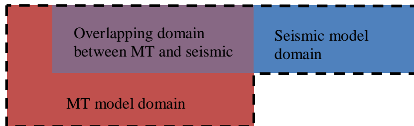
Figure 2-10: The different between MT and seismic model domains, which may cause problems for joint and co-operative inversion of MT and seismic data
