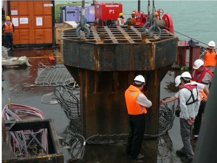
Figure 3-5: First application of a double sided DC-DR grater pounder in the world
