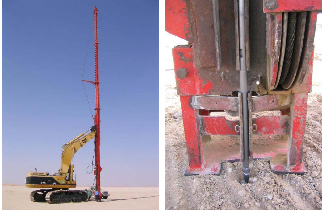
Figure 3-29: Quick probing machine composed of an excavator base, a mast and a penetrating tubular rod.
