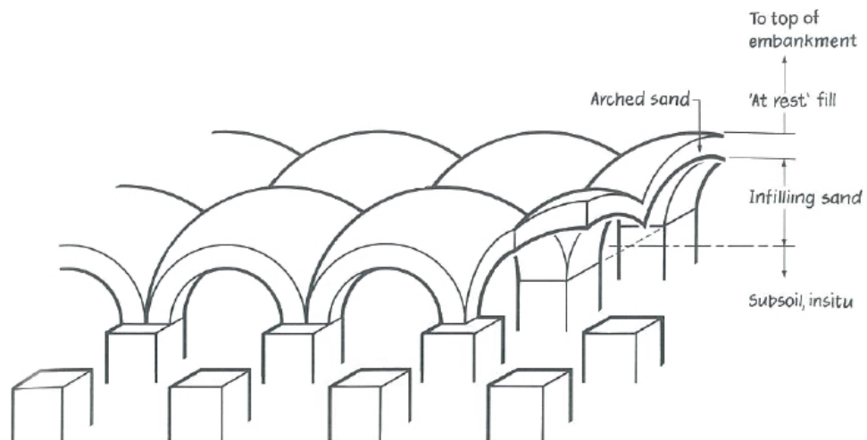
Figure 2-82: Isometric view of a grid of pile caps (DR columns) and a series of domes forming vaults spanning between them (Hewlett and Randolph, 1988)
