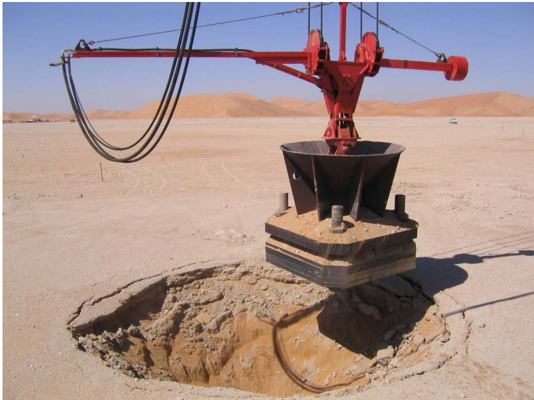
Figure 3-24: Automatic grabbing of a 35 ton poulder by MARS
