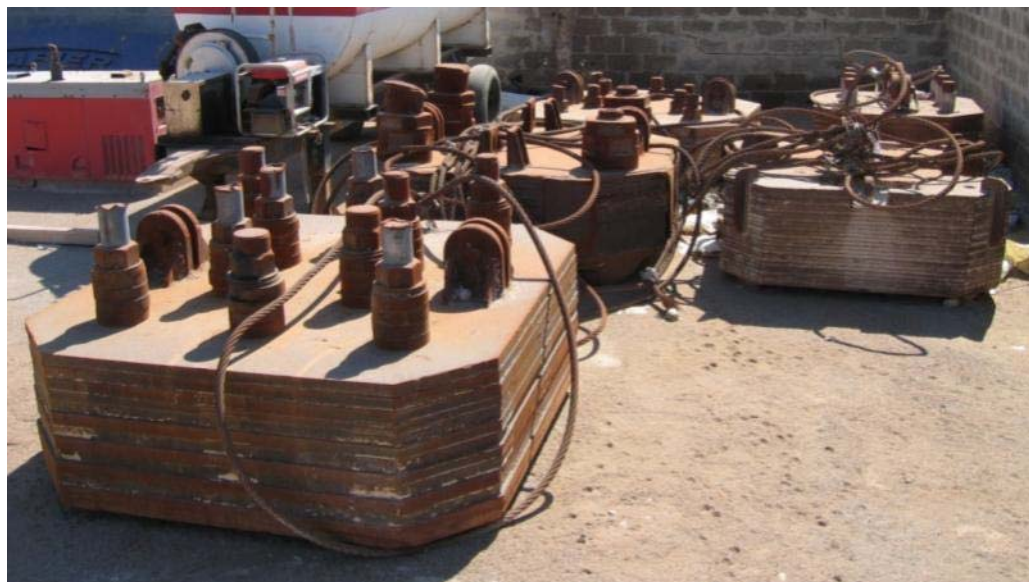
Figure 2-113: steel pounders composed of steel plates
