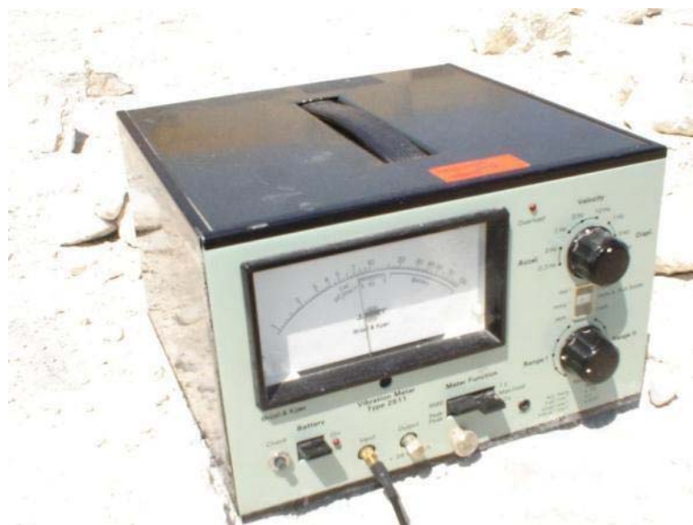
Figure 2-134: Vibration metre for measuring peak particle velocity
