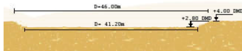
Figure 3-199: Cross section of excavation for reaching working platform level
