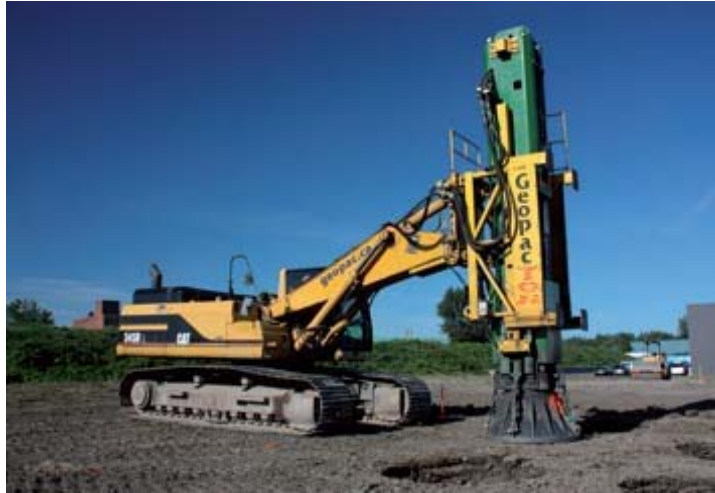
Figure 2-115: Rapid Impact Compactor
