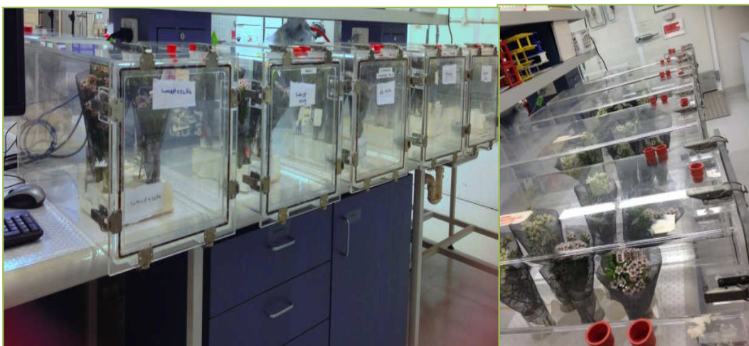
Figure. 3.4. Application of ethylene treatment ( 10 \mu\text{L L}^{-1} ) by injecting pure ethylene into glass chambers containing waxflower stems for 24 h. Flowering stems were placed in mesh cones inside the glass chambers prior to injecting the pure ethylene using a 1ml syringe inserted through a rubber port located at the top of each chamber (Seaton, 2006).
