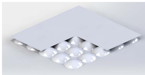
198 199 Figure 7. Grid sphere dome sandwich structure with top plate partially removed for 200 illustration.
