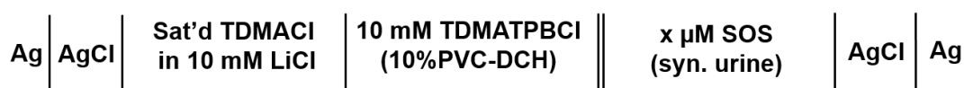
Scheme 5.2.1 Schematic representation of the electrochemical cells employed, where x represents the sulfated carbohydrate (e.g. SOS) concentrations utilized in the study.
