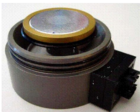
Figure 3.8: Typical Rotating Stage with Uniform Deposit in centre of aluminium foil substrate (MSP Corporation, 2017).
