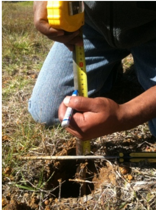
Figure 3:11 - Marking out 15cm for depth of cylinder to collect sample
