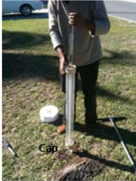
Figure 3:6 – Installation of the Guelph Permeability Test Kit
