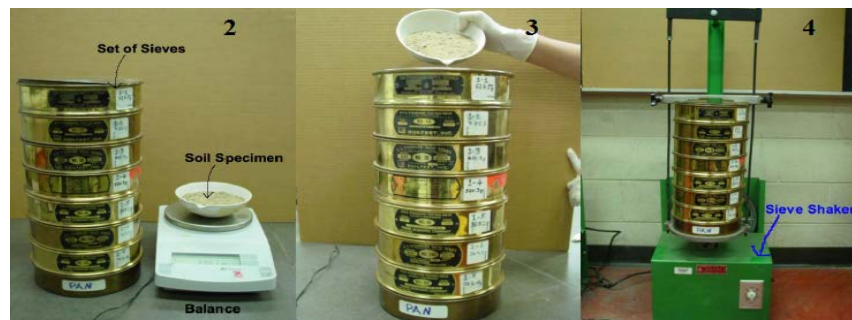
Figure 3:17 - Sieve Analysis step by step test procedure
