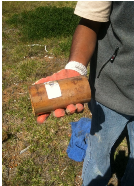
Figure 3:13 – Collecting a sample in clayey soil condition
