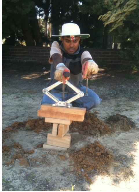
Figure 3:13 – Collecting a sample in clayey soil condition
