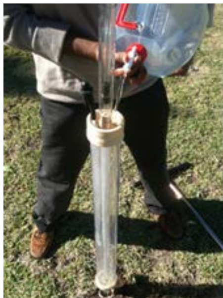
Figure 3:7 - Filling the outer and inner reservoirs
