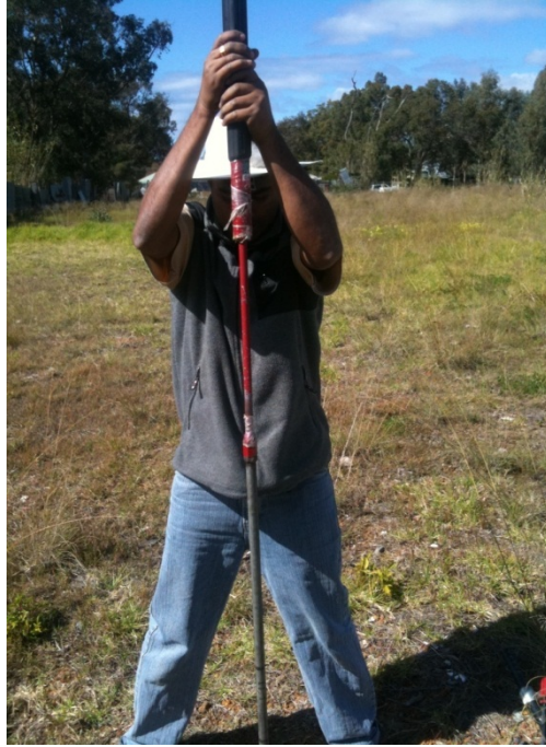
Figure 3:12 - Collecting the sample by hammering
