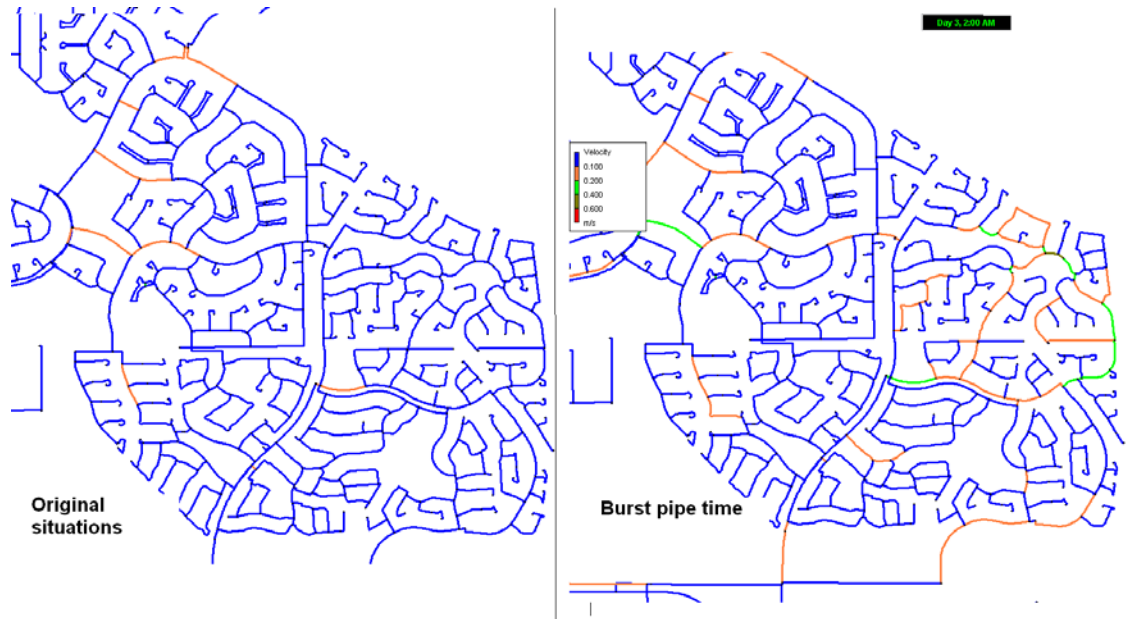
Figure 8.3: PSM velocity before (left) and during burst pipe event at suburb A.
