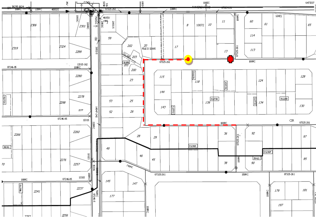
Figure 10.3: Site 4aD, loop pipe or dead-end, unidirectional flow length = 376 m; Tank 2 supplies the water. Note the closed valve was not working during fieldwork.
