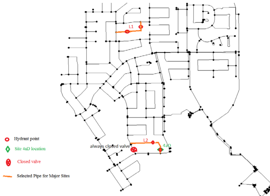
Figure 9.1: The locations of selected pipes (L1 and L2) for major sites of fieldwork.
