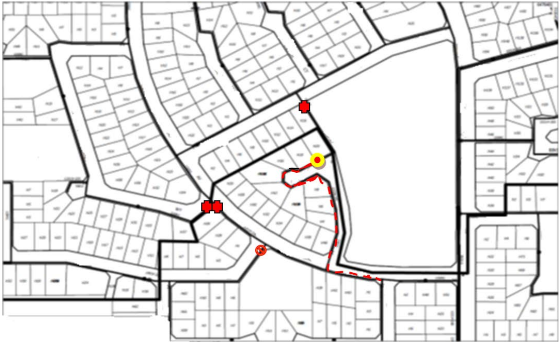
Figure 10.1: Site 1aH, dead-end pipe; unidirectional flow length = 324.2 m; Tank 1 supplies the water.
