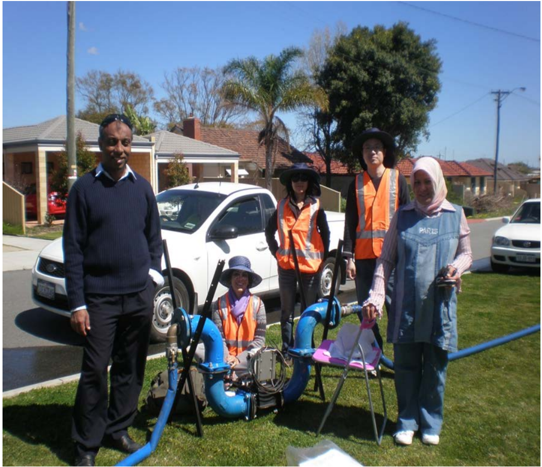
Figure 9.5: Mag flow meter “AquaMaster™” connected at site Ma1.
