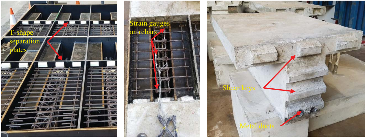
Fig. 3: Casting of specimens
