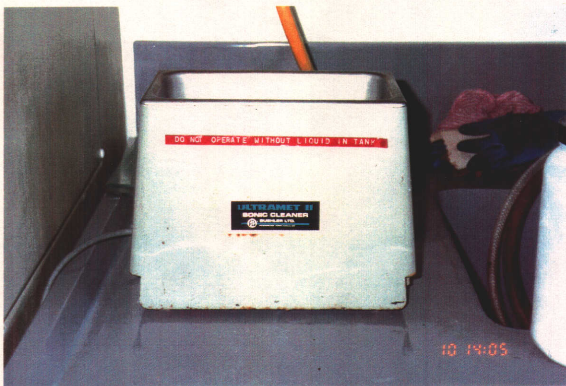
Figure 3.8. Ultrasonic bath used in polished section preparation.
