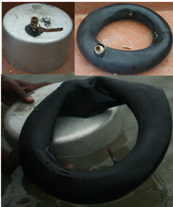
Fig. 6. Seepage meter used to measure the SGD.
