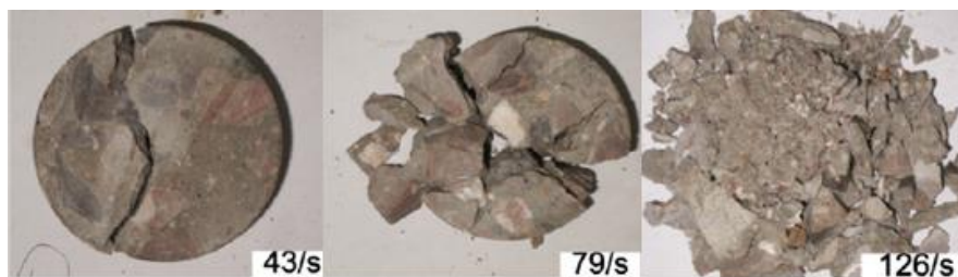
482 Fig. 12. Failure mode of unconfined concrete specimens under different strain rates [22].
