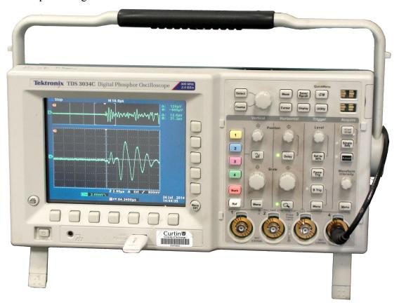
Figure 11. Digital oscilloscope (Tektronix TDS 3034C), capable of recording 10000 equally spaced time samples with maximum frequency of 300 MHz and 512 level averaging.
