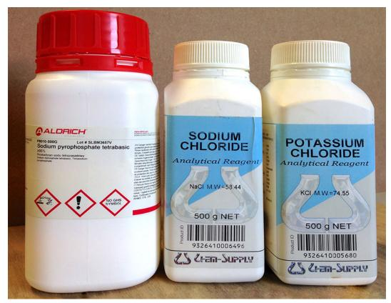
Figure 7. Chemicals used for the preparation of silt-clay mixtures with a desired clay microstructure.
