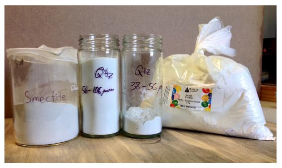
Figure 2. Mineral powders used for preparation of clay-silt mixtures.
