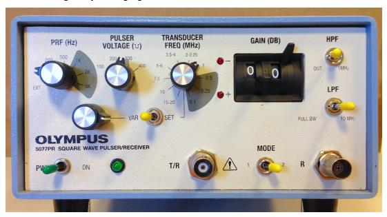
Figure 10. Square wave pulser/receiver (Olympus 5077PR) used for excitation and registering of ultrasonic pulses with typical setup parameters shown.
