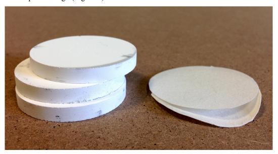
Figure 8. Porous alumina plates (25% porosity) and filter paper (2.5  $\mu$ m pore size) used to hold the clay-silt mixtures inside the oedometer.
