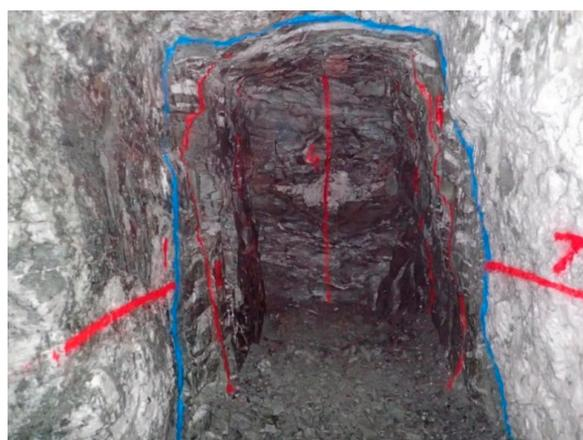
**Figure 3.** Orientation of linear samples (e.g., chip-channel) to match geological requirements. Sub-vertical quartz reef in foreground with area of flat veining on the footwall (blue line marks footwall contact). Sub-vertical reef sampled horizontally (samples 1 and 7), whereas flat footwall veins sampled vertically (samples 2–6).
