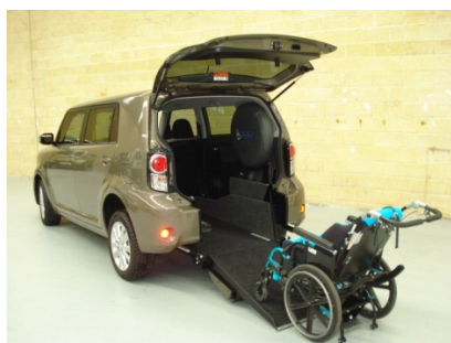
Example of a rear wheelchair access vehicle modification. Used with kind permission from Freedom Motors Australia Pty Ltd (26/7/11).
