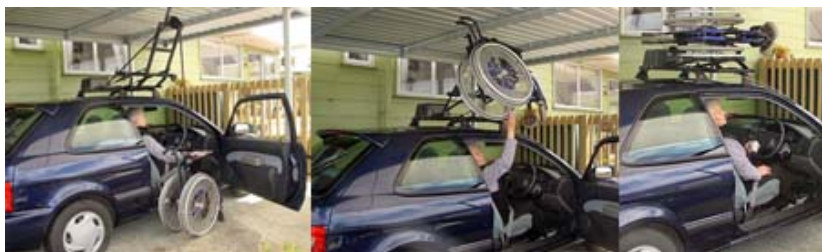
Example of a car rooftop hoist system. Used with permission from IKON Engineering Development Ltd (26/07/2011).
