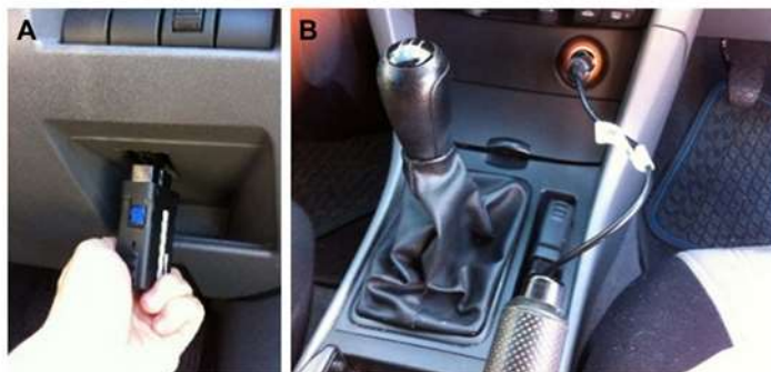
Figure 3 In-vehicle driver monitoring device inserted either into the On Board Diagnostic II (OBD II) port of the vehicle (A) or the cigarette lighter (B).
