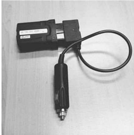
Figure 7. In-vehicle monitoring device used to measure naturalistic driving behaviour
