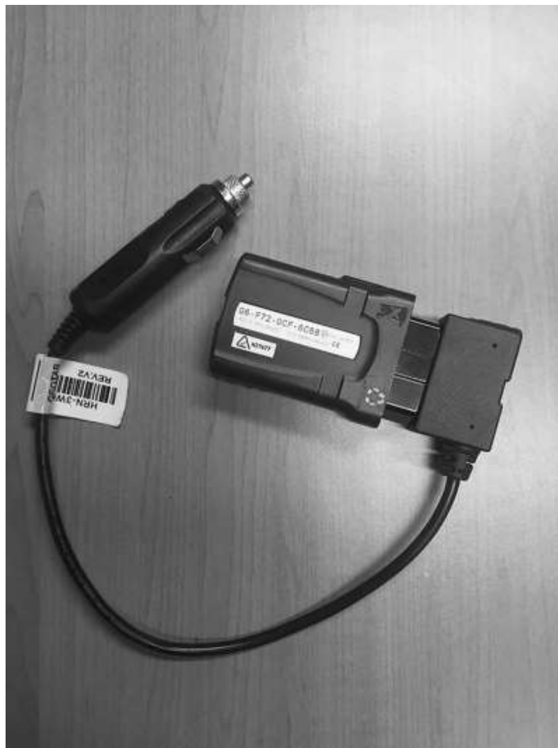
Fig 1. In-vehicle driver monitoring device.
