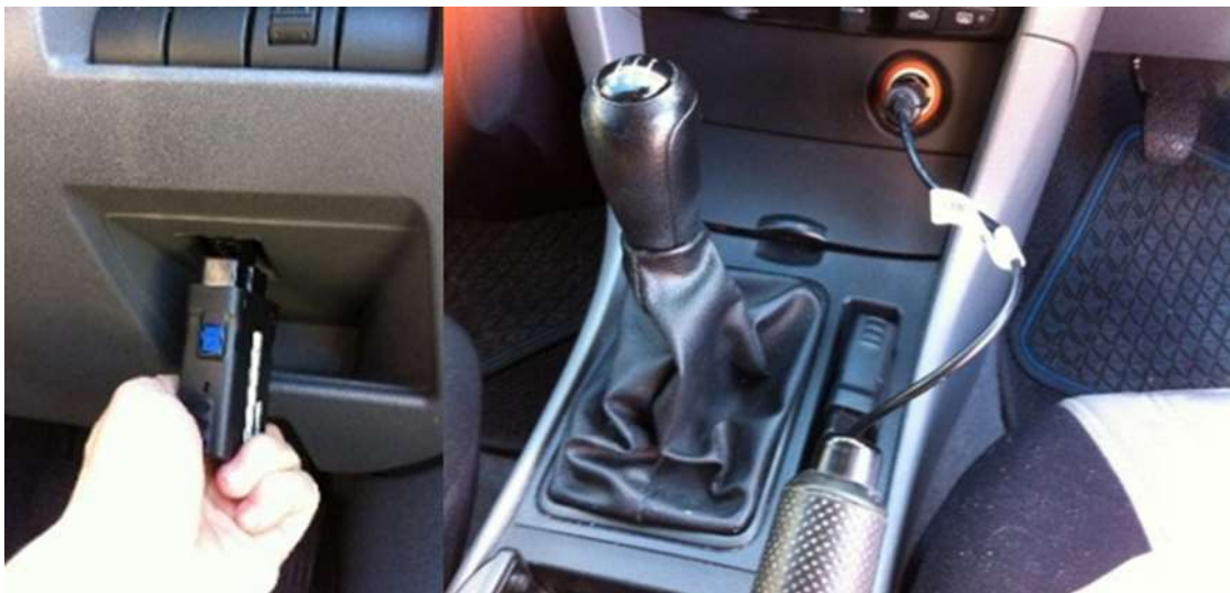
Figure 8. In-vehicle monitoring device connected onto OBD II port (left) and the cigarette lighter (right)
