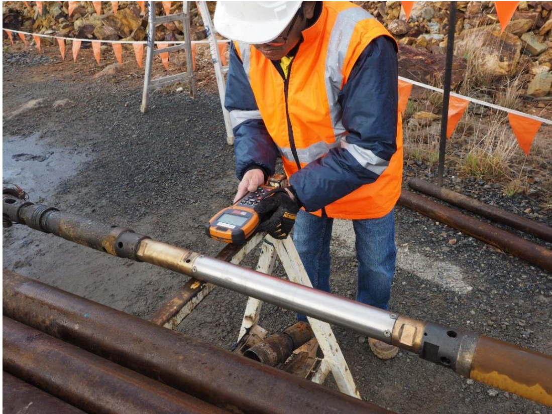
Figure 4-2 An example of the Auto-shuttle being tested in another hole nearby (as this thesis was being written). The Auto-shuttle is located between the back-end-assembly on the left and the inner tube on the right. The operator in the photograph is downloading the raw data from the Auto-shuttle, which is then uploaded to a PC for processing.
