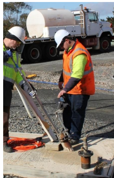
Figure 4-3 Our spectral gamma sonde assembly lying on the ground (foreground left) and being deployed at Brukungu in hole RD01 (right).
